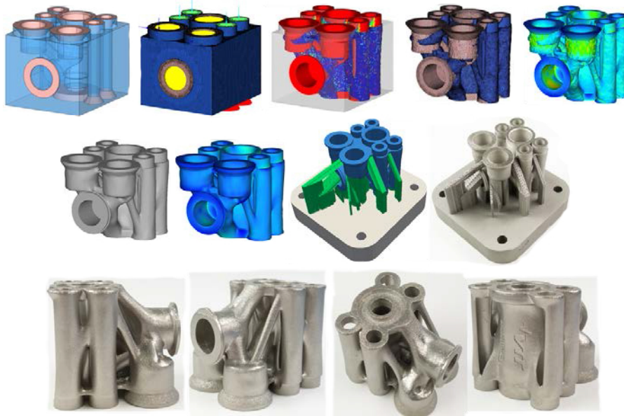
Figure 1. Process for designing a hydraulic valve block specifically for AM, including topology optimization, results interpretation, smoothing of design, design validation, and print preparation [8].
