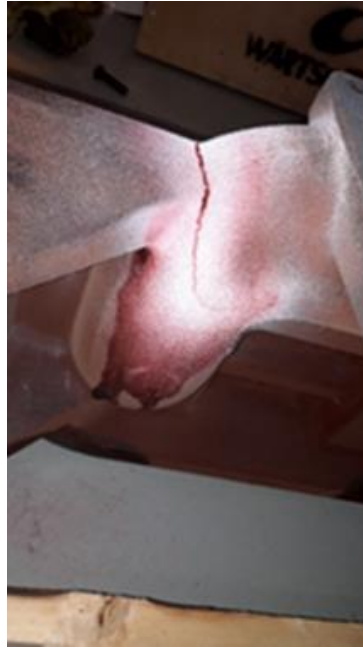
Figure 1. Low-cycle thermal fatigue caused exhaust support failure.
