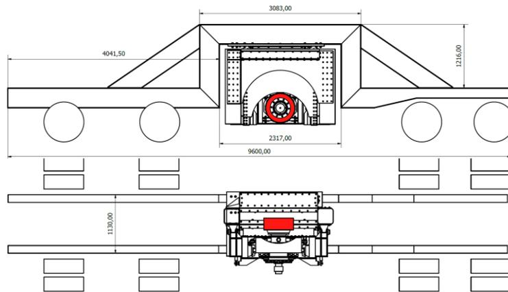
Figure 1. Schematic view of the trailer. The measured tyre wheel is annotated with red color.
