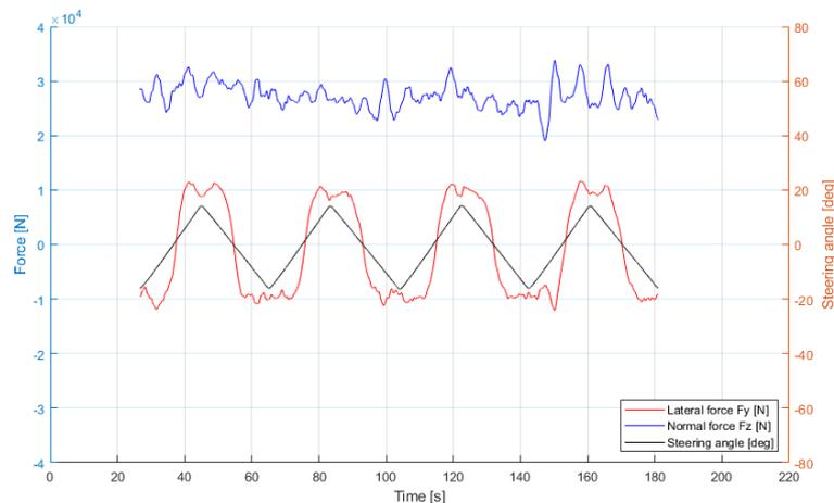
Figure 4. Filtered lateral and normal forces with steering angle in time domain for the 4 full sweeps of the test run.
