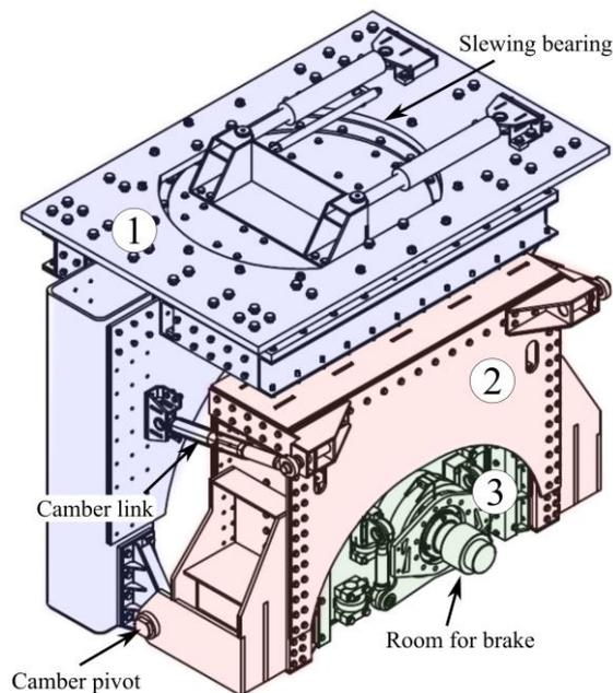
Figure 2. The main components of the measurement system.
