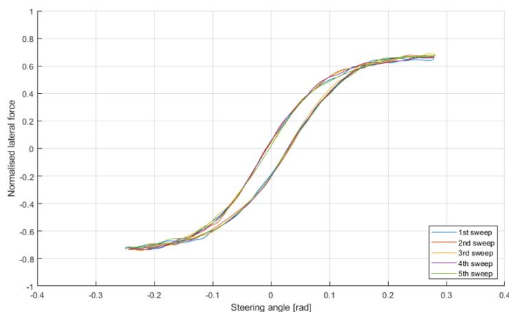
Figure 9. Individual sweeps of pure lateral force test run in wet asphalt with normal force of 39829 N.
