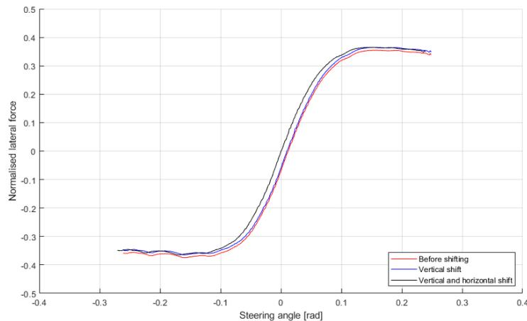
Figure 7. Elimination of lateral force curve shift caused by tyre conicity, ply-steer etc.
