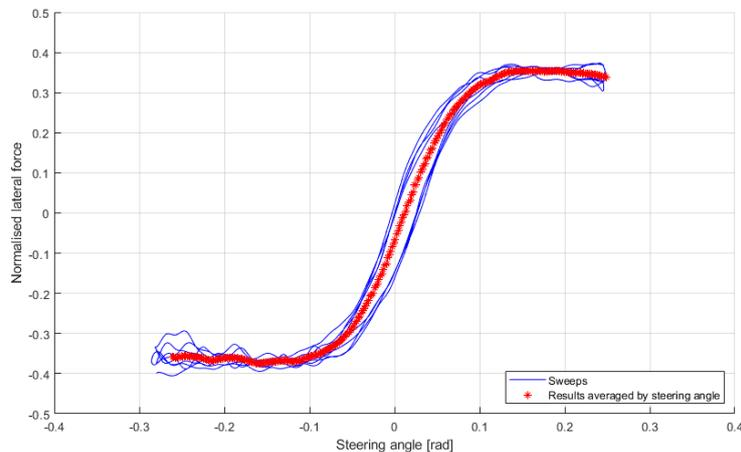
Figure 6. Relaxation compensation for the normalized lateral force curve.
