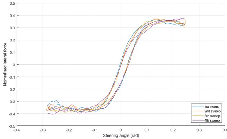
Figure 5. Normalized lateral force curves as a function of steering angle separated to individual sweeps of the measurement run.
