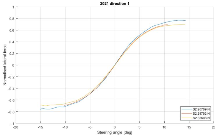
Figure 10. Pure lateral slip force curves of "S2" tyre on wet asphalt.
