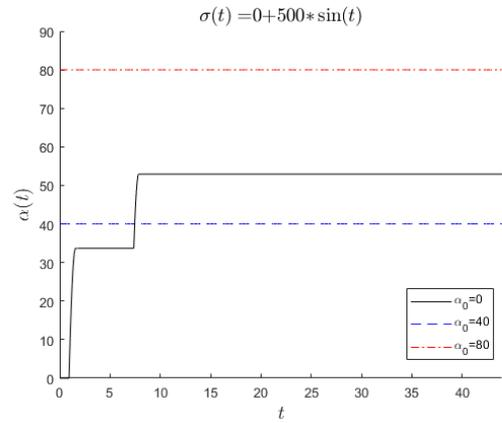
Figure 6. Back-stress  $\alpha$ ; maximum lifetime  $N_f = 2567297$  with  $\alpha_0 = 80$  MPa
