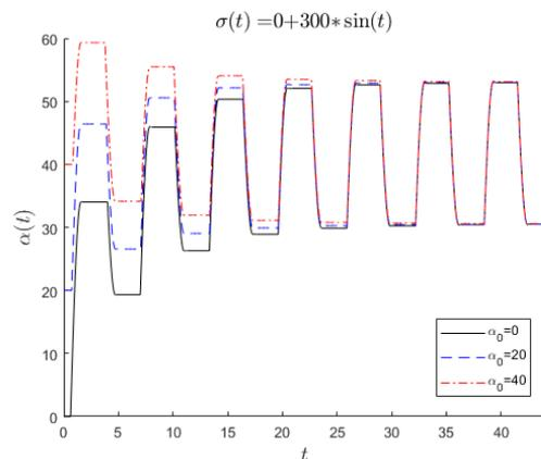
Figure 2. Back-stress  $\alpha$ ; maximum lifetime  $N_f = 163462$  with  $\alpha_0 = 40$  MPa
