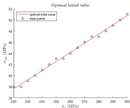
Figure 21. The optimal initial value curve, dataset S45C
