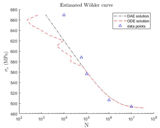
Figure 20. Estimated Wöhler curve with optimal initial value
