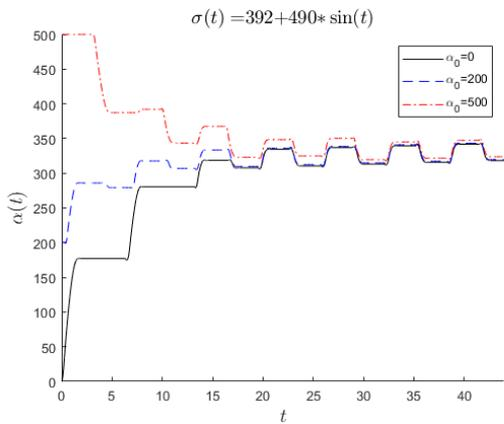
Figure 12. Back-stress  $\alpha$ ; maximum lifetime  $N_f = 97850$  with  $\alpha_0 = 500$  MPa
