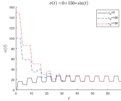
Figure 14. Back-stress  $\alpha$ ; maximum lifetime  $N_f = 260777$  with  $\alpha_0 = 150$  MPa
