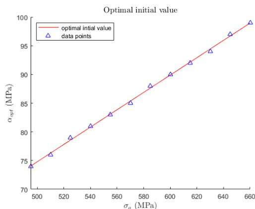
Figure 22. The optimal initial value curve, dataset SAE 4340
