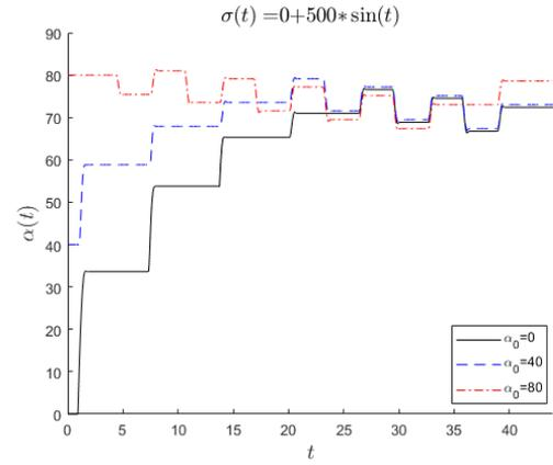
Figure 8. Back-stress  $\alpha$ ; maximum lifetime  $N_f = 6170373$  with  $\alpha_0 = 40$  MPa
