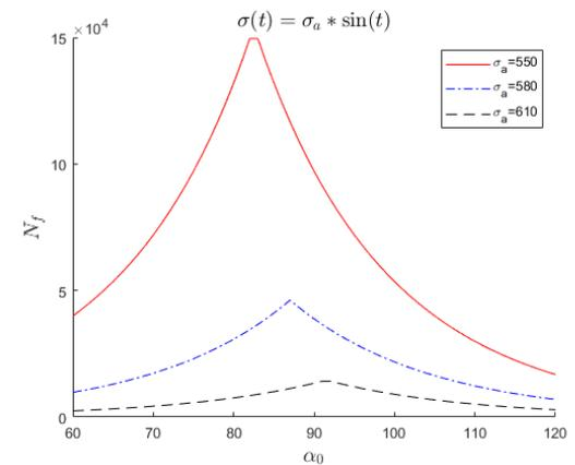
Figure 18. Lifetime dependence on initial value, dataset SAE 4340
