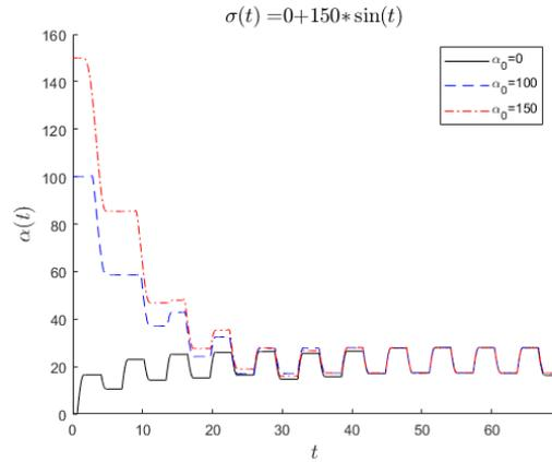
Figure 16. Back-stress  $\alpha$ ; maximum lifetime  $N_f = 272618$  with  $\alpha_0 = 0$  MPa
