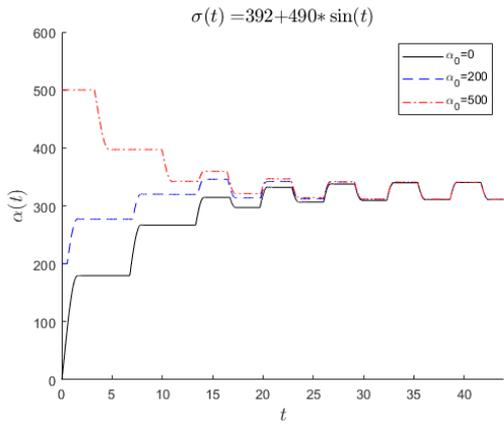
Figure 10. Back-stress  $\alpha$ ; maximum lifetime  $N_f = 105309$  with  $\alpha_0 = 200$  MPa
