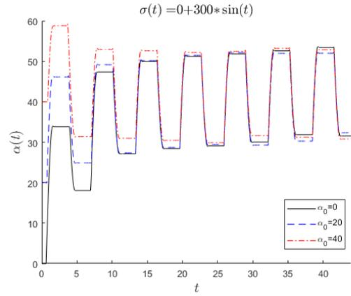
Figure 4. Back-stress  $\alpha$ ; maximum lifetime  $N_f = 162662$  with  $\alpha_0 = 40$  MPa
