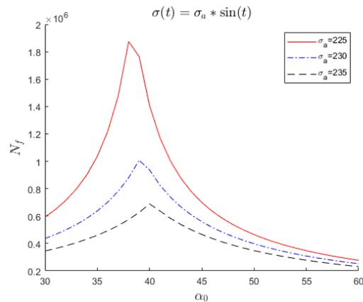
Figure 17. Lifetime dependence on initial value, dataset S45C
